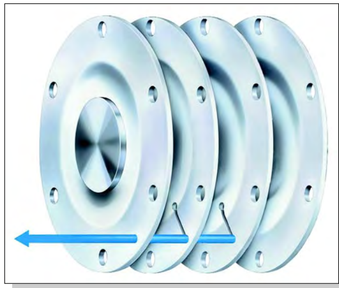
Figure 2. Four layer PTFE sandwich diaphragm pack with one operating diaphragm, two monitoring diaphragms with signaling channels and one back-up diaphragm.
