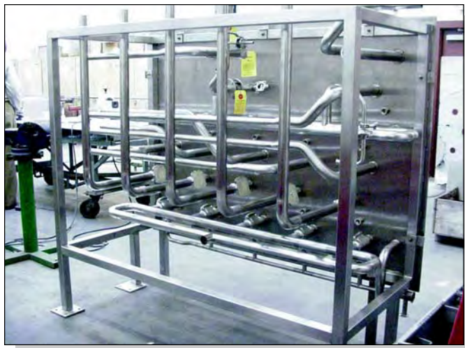
Figure 8. Recessed self-supporting frame panel.
