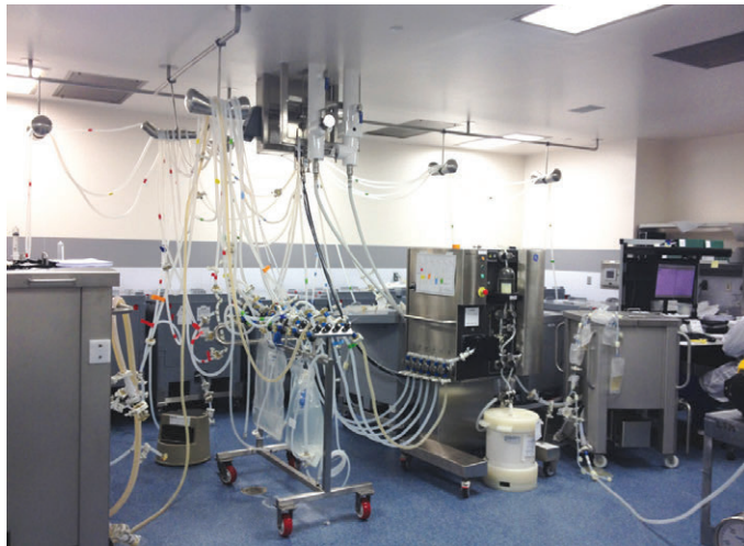
Purification single-use chromatography in operation.
