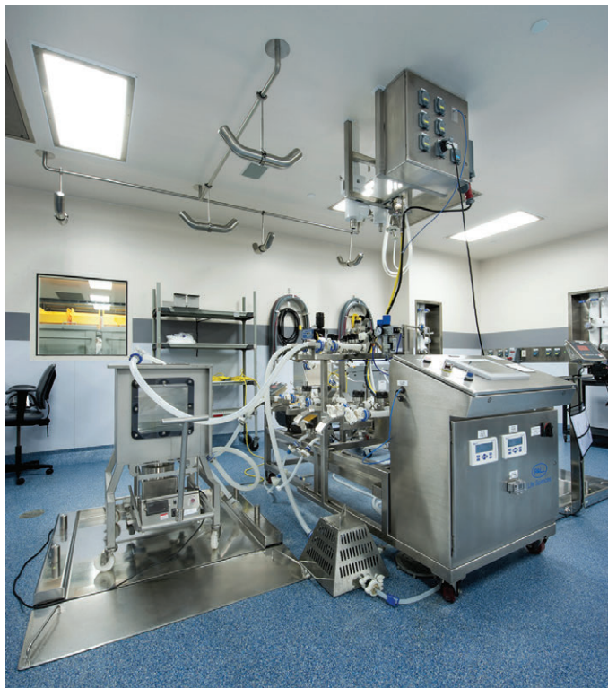
Single-use ultrafiltration skid.
