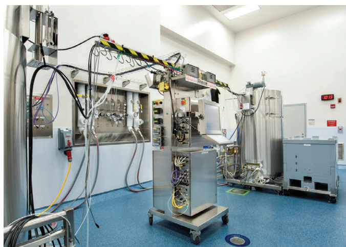
Cell culture single-use bioreactor with utility panel.
